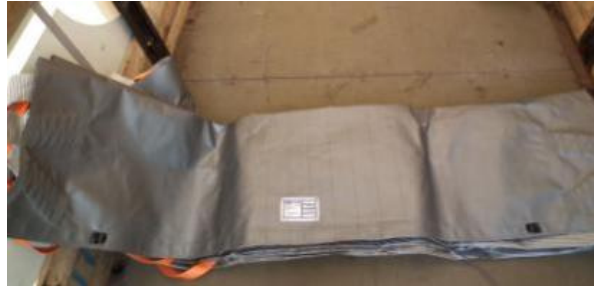
Figure 16. Spread out the Fix fabric with the tag to the rear of the trailer.
