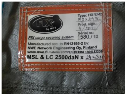
Figure 17 & 18. Tag for the type code tells (from top down) the size and model of the cover, production month and year, serial number, DEKRA approval number, number of straps and strap length. Tag for strap tells breaking strength BS, lashing capacity LC, material, length, applied standard and manufacturer.
